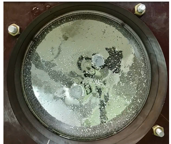
Figure 2. Electrovortex flow in the bowl with two submerged electrodes visualized by hydrogen bubbles. I = 800 A.
